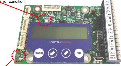
Light sensor facing forward is used to dim the LED signs or the backlight of LCD signs. You may alter the behaviour of dimming through the DISPLAY menu.
